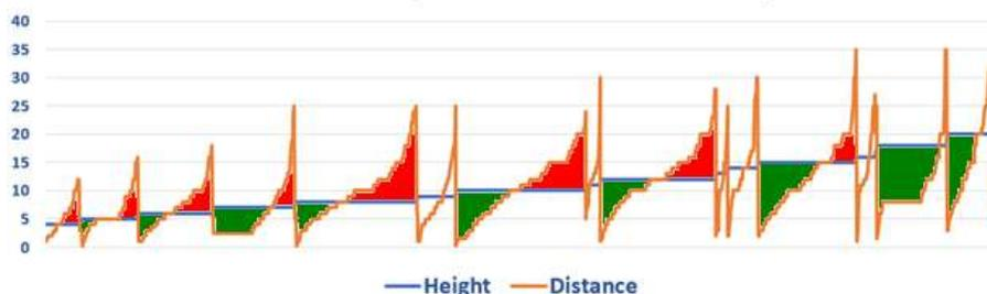
In contrast, the willow (above) appears to have more extensive root cover as illustrated by the areas shaded red, illustrating where the distance to the damage exceeds the tree height.
