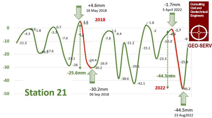
At Station 21, above, 30.2mm of subsidence was recorded in 2018 between May and September (readings are generally taken at two-month intervals), and 44.5mm between April and August 2022. 2019 and 2020 have similar values.
