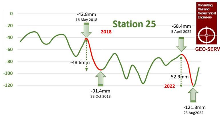
At Station 25, 48.6mm of subsidence was recorded from May to October in 2018, and 52.9mm between April to August in 2022. Movement in the intermediate years was 42.3mm in 2019, 30.5mm in 2020 and 8.3mm in 2021, reflecting the problems associated with predicting the risk of root induced clay shrinkage. The interval between readings varies by year and the above are approximations only.
