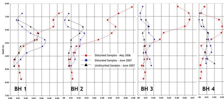
Oedometer test results from boreholes sunk in May 2006 (red) and June 2007. BH 3 is nearest level station 7 in the top graph.
