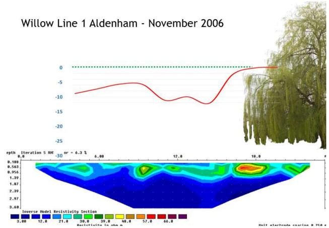
Recovery of around 20mm was recorded at the station where maximum subsidence had taken place, and the ERT image shows a reduction in resistivity.
