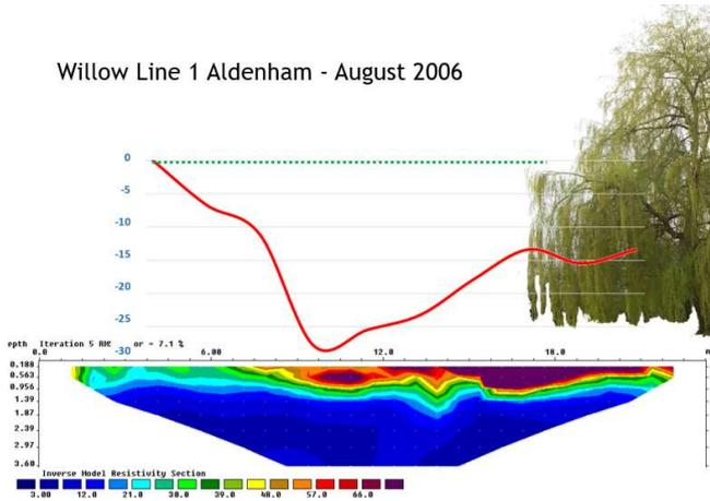
The zone of desiccation is identified by the precise levels, and maximum movement coincides with the red/yellow/green zones shown on the ERT plot.
